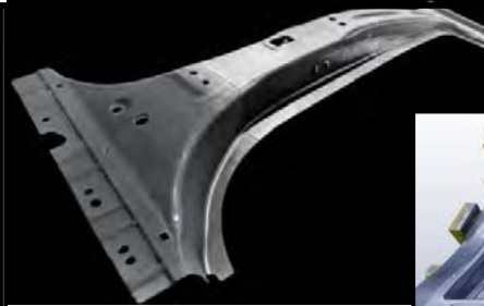
Press forming – tooling and formed sheet metal (car inner wing)
